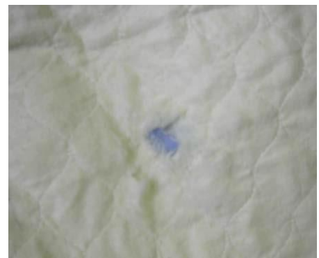
Shifting of thermal liner material (batting)
