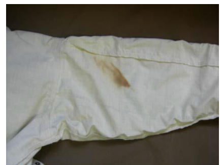
Discoloration on moisture barrier caused by thermal damage
